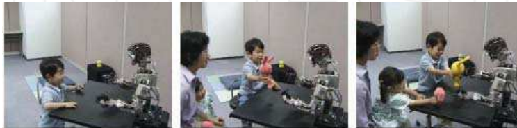
Fig. 8. Unfolding interaction between Infanoid and a four-year-old boy: neophobia (left), exploration (middle), and interaction phases (right).
